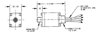
Figure 1 182P Vacuum Switch
